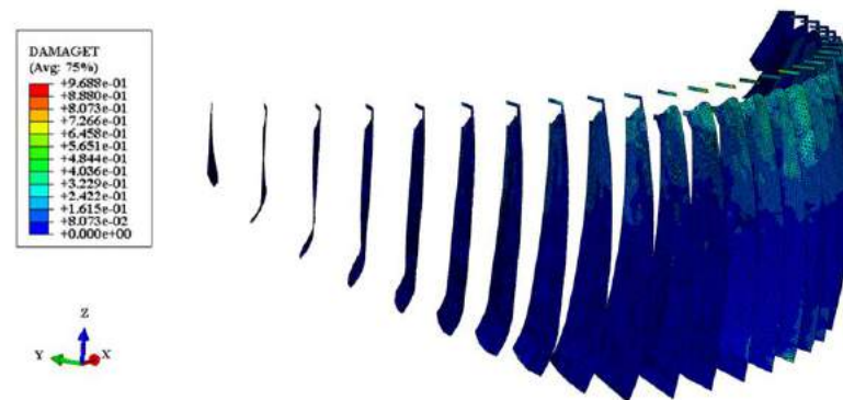
Figure 1. Tensile damage parameter T [-], under Accumoli (RI) seismic event, with the normal reservoir level condition.
