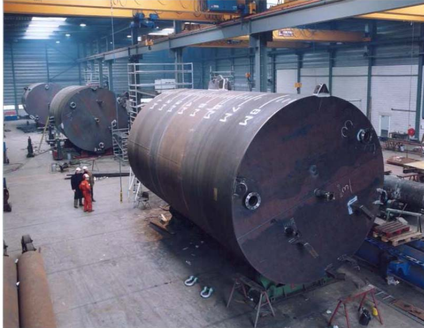
Figure 1. (a) Caisson in fabrication yard (after Tran, 2005).
