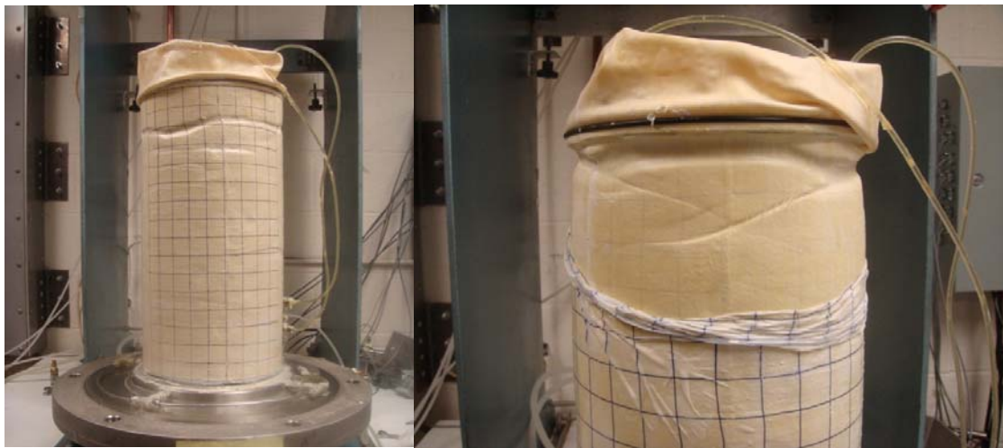
Fig. 9. Shear band pattern in hollow cylinder specimen with (a) \alpha = 67.5^\circ and b = 1.0 and (b) \alpha = 90^\circ and b = 1.0 . In the latter case, the outer layer of the membrane has been peeled off to clearly show the width and the sides of the “canyon” shear band oriented horizontally in the direction of the major principal stress.
