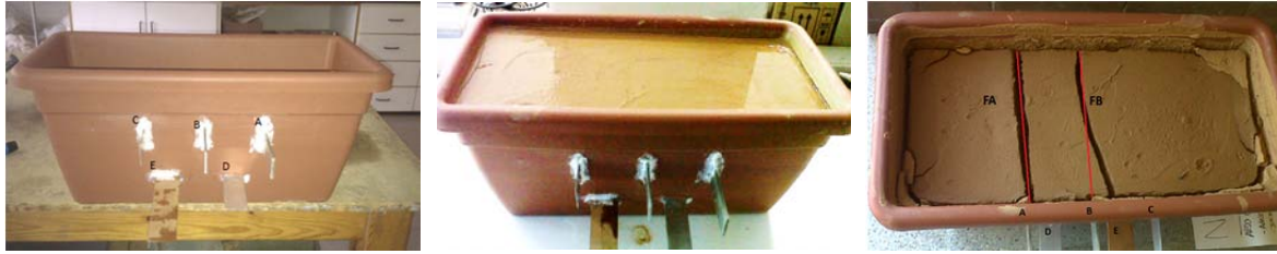
Fig. 3. Block test: (a) mold with strips inserted; (b) after pouring slurry; (c) surface cracks at 30 days
